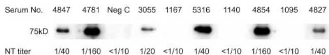
FIG. 1. Baculovirus-expressed H5 antigen from A/Vietnam/1203/04 purified by affinity chromatography columns (Protein Sciences Corporation, Meridian, CT). One microgram of H5 protein per lane was separated on a 10% sodium dodecyl sulfate-polyacrylamide gel and immunoblotted with pig sera at a dilution of 1/200. Horseradish peroxidase-conjugated anti-pig immunoglobulin (DakoCytomatron, Glostrup, Denmark) was used at a dilution of 1/10,000 as recommended by the manufacturer. All the sera giving positive neutralization test reactions and a random selection of sera giving negative neutralization test results were tested by Western blotting. A representative result is shown.
